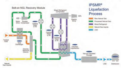
Chart proprietary IPSMR process technology is less complex than dual mixture process and provides process optimization for liquefaction of natural gas, ethane, propane, butane and air.
