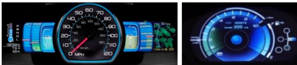
Figure 217: Examples of LCD Instrument Clusters 152
