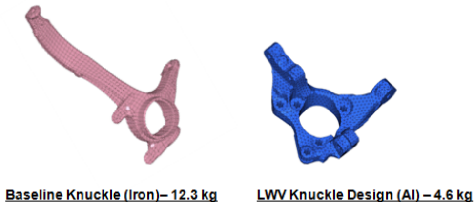
Figure 202: Steering Knuckle – Baseline and LWV Design
