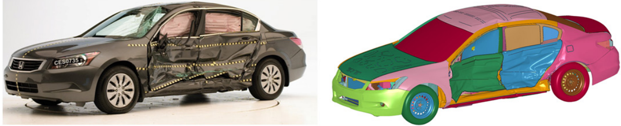
Figure 19.5- 2: Post-crash views of Honda Accord 2011 and light weight vehicle after IIHS side barrier test
