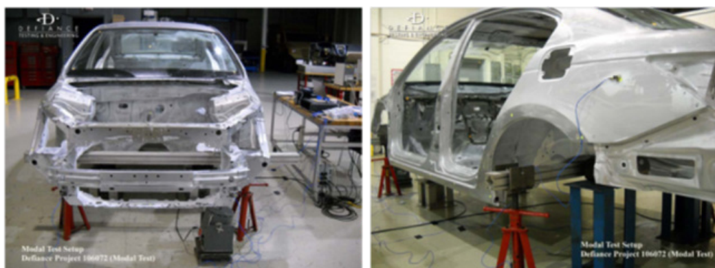
Figure 43: Vehicle Set-Up for Normal Modes Test
