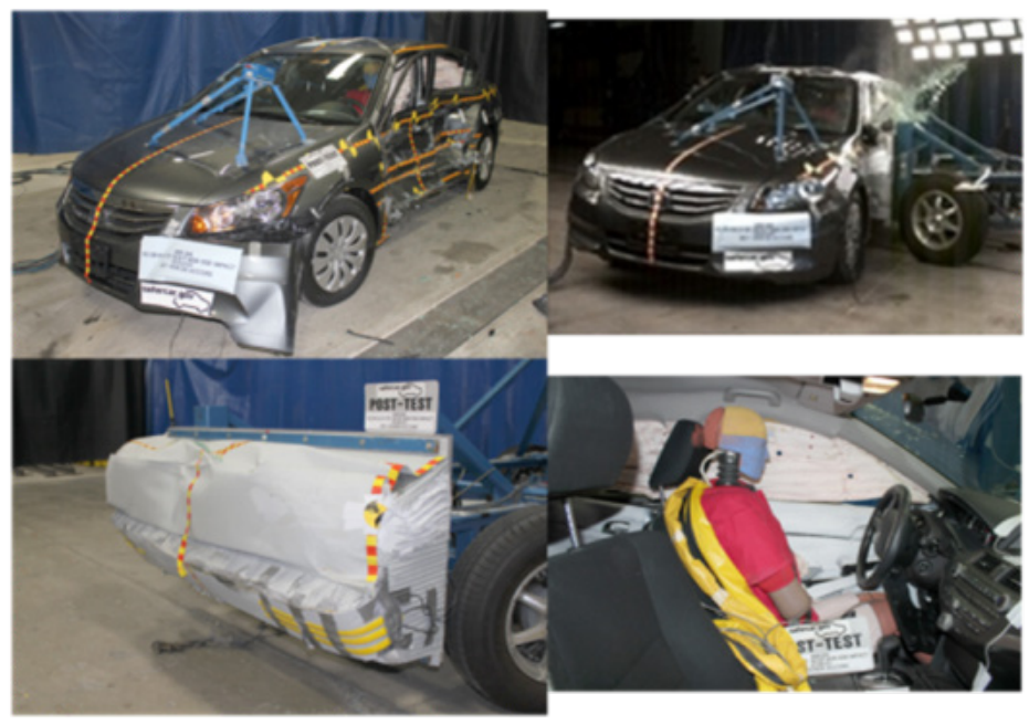
Figure 60: Test set up and the post-crash vehicle of the NCAP side impact test with moving deformable barrier 66
