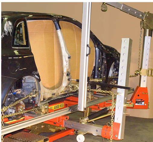
Figure 136: Straightening of a b-pillar in a repair rig
