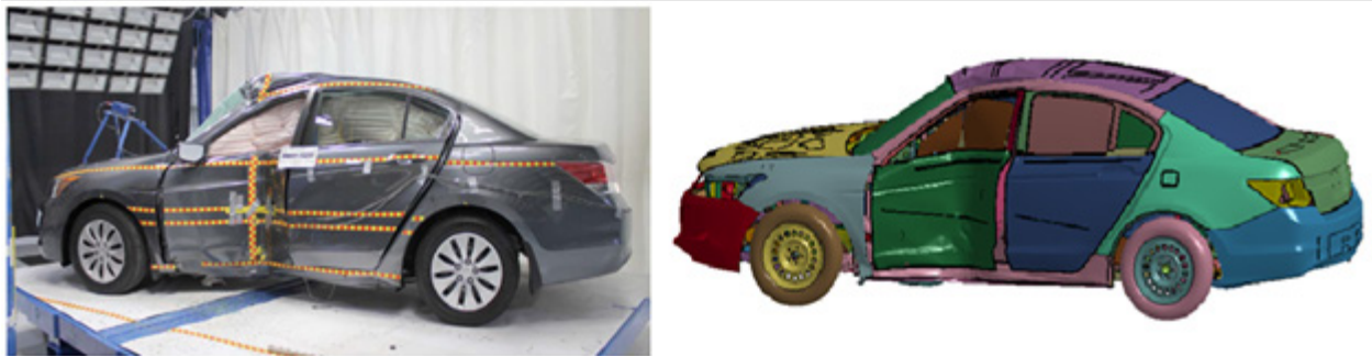
Figure 19.3- 2: Post-crash views of Honda Accord 2011 and light weight vehicle after NCAP side pole test
