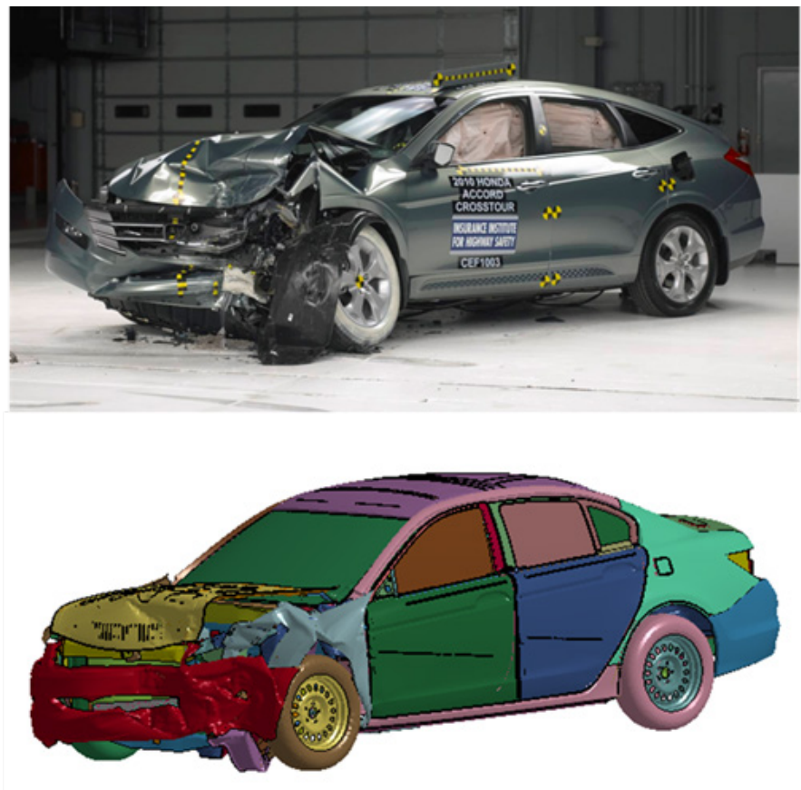
Figure 309: Post-crash vehicles for the MY 2011 Honda Crosstour actual laboratory crash and the simulation for LWV in the IIHS 40% offset frontal test
