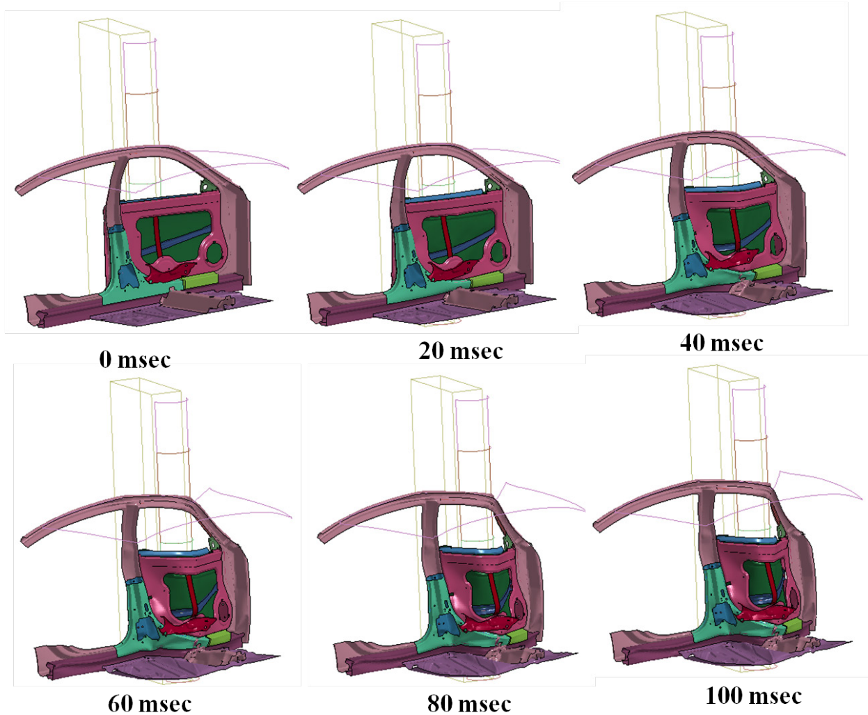
Figure 19.3- 4: Crush of six key structural parts over the time of the NCAP side pole test
