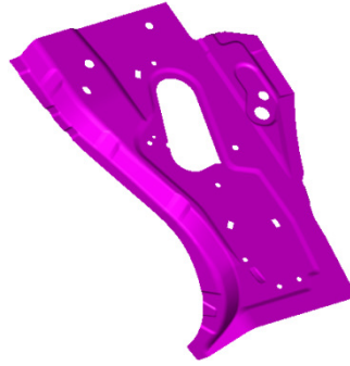
Figure 331: Typical part, B-Pillar inner lower, stamped in a tandem press line
