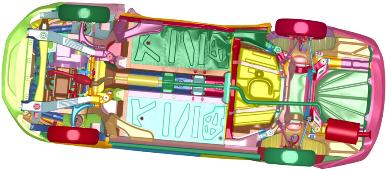
Figure 19.5- 7: Bottom view of light weight vehicle after IIHS side barrier test
