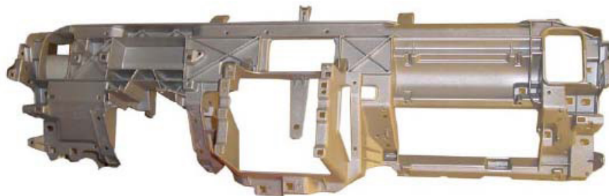
Figure 215: Cast Magnesium I/P Beam (GM Epsilon shown)
