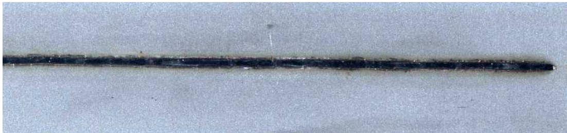
Figure 477: Weld Seam with 0.20 mm Gap between the zinc coated welded panels 241
