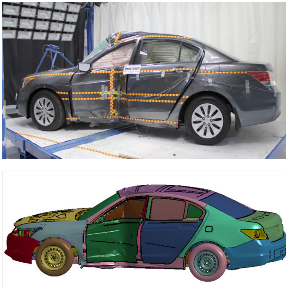
Figure 280: Post-crash vehicles for the actual laboratory crash and the simulation in lateral pole test
