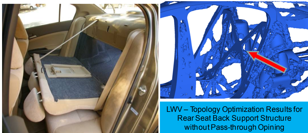
Figure 93: Topology Optimization Results – Rear Seat Back
