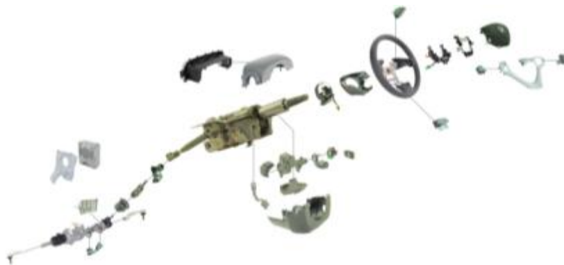
Figure 27: Components That Make Up the Steering Subsystem 29
