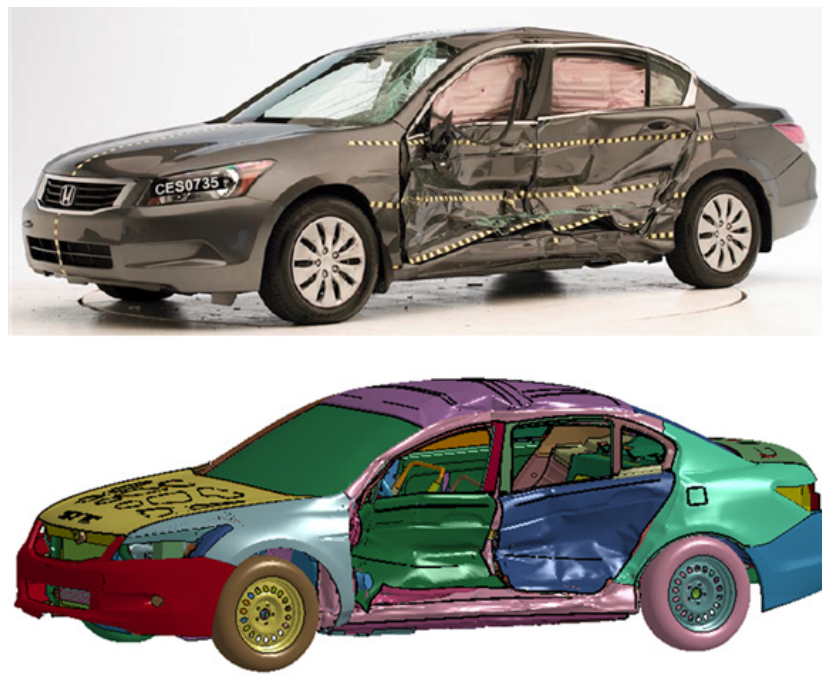
Figure 298: Post-crash vehicles for the actual laboratory crash and the simulation in IIHS lateral impact test
