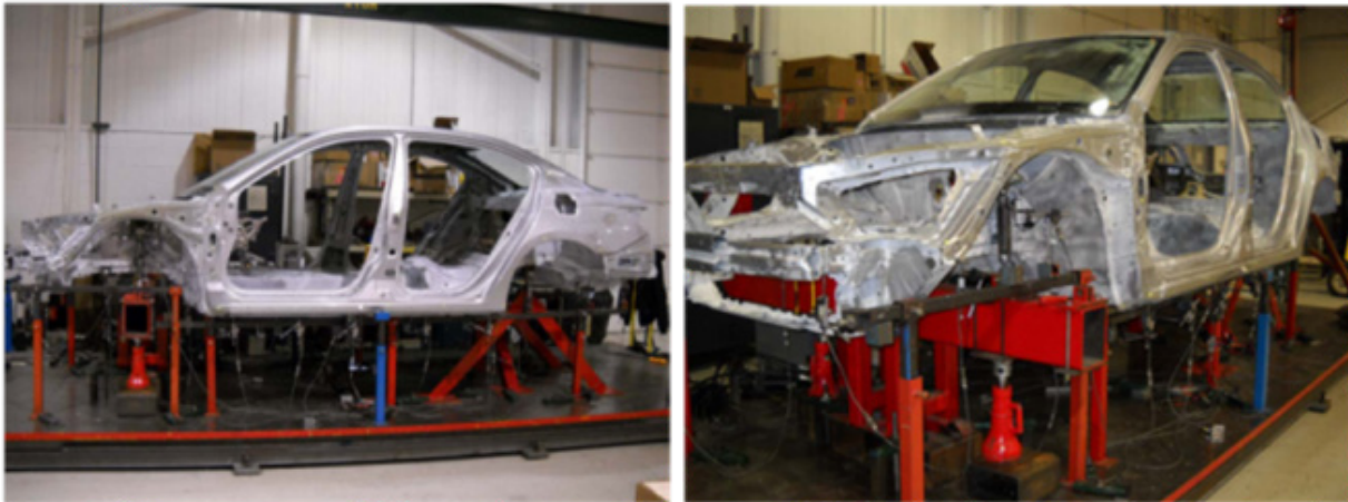
Figure 46: Body Structure on Test Rig for Torsion and Bending Stiffness Test
