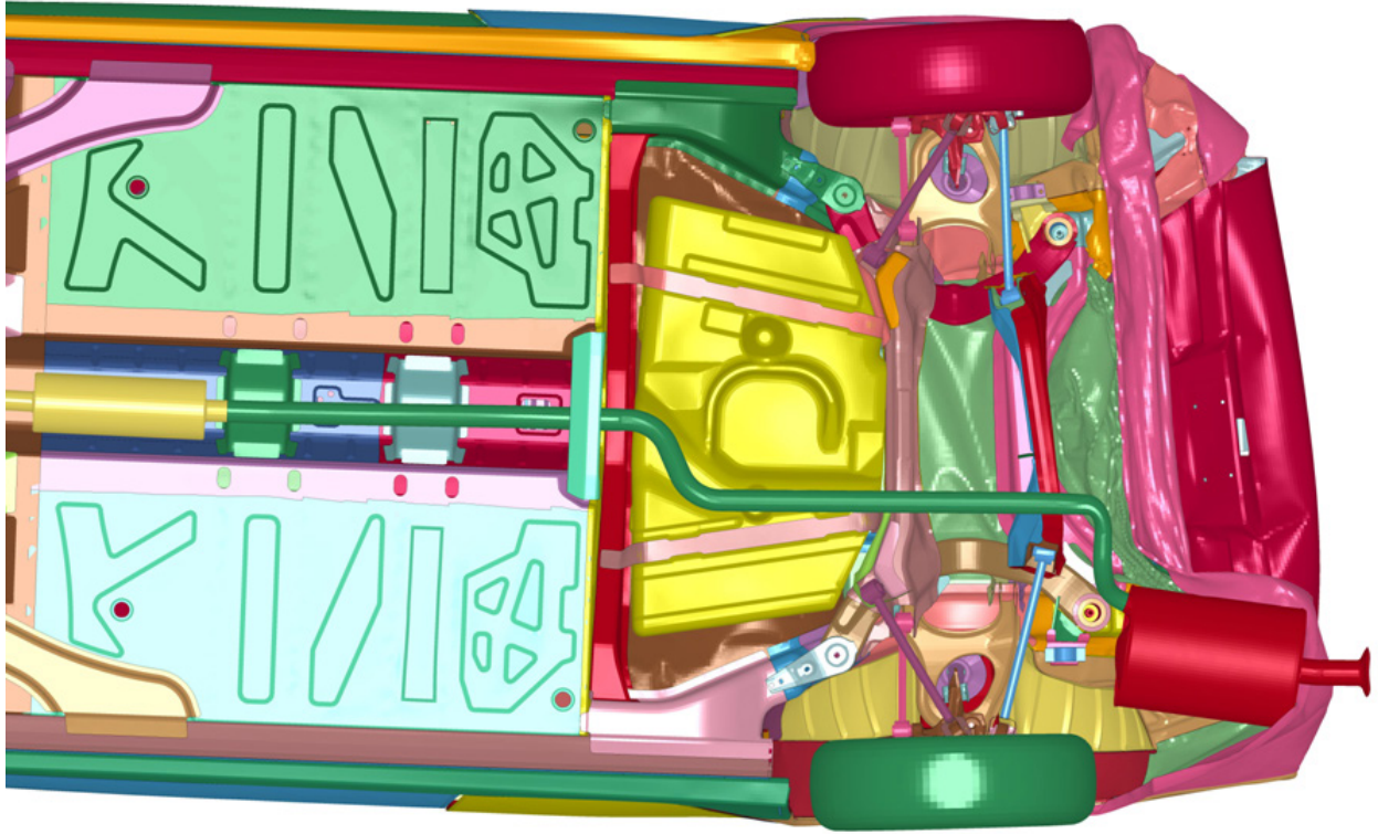
Figure 19.7- 4: Bottom view of light weight vehicle after FMVSS No. 301 test
