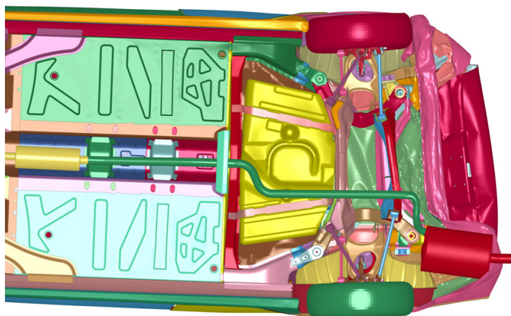
Figure 320: Bottom view of LWV after FMVSS No. 301 test
