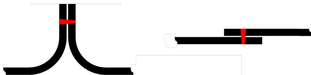
Figure 483: Schematic representation of a flange weld (left) and a lap joint weld (right)
