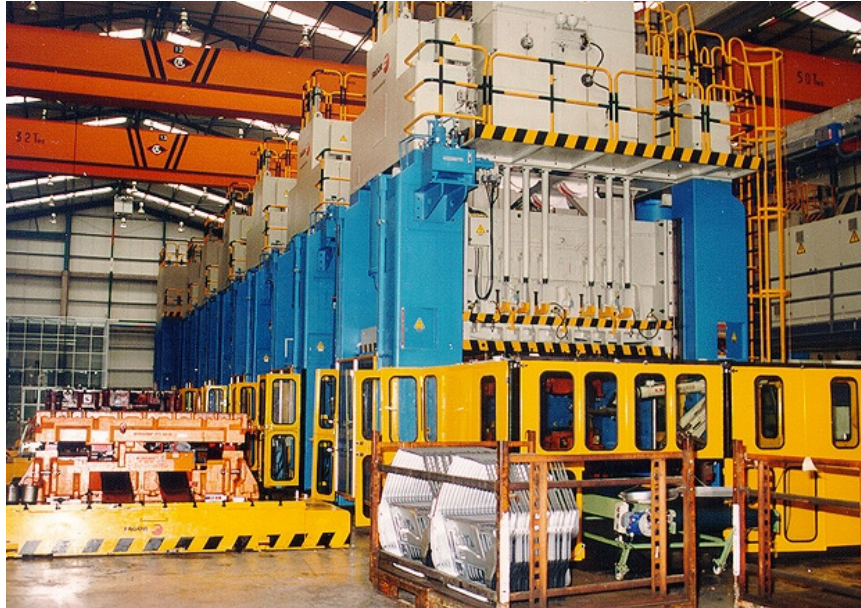
Figure 333: Typical Transfer Press Line for a door inner panel.
