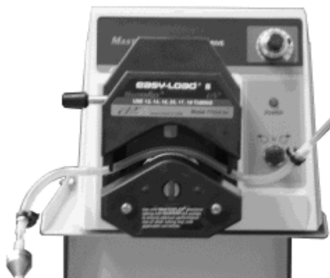
Figure 11. Sample pump with pump head raised and tubing in place
