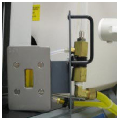
Figure 9. Zinc selenide flow-through cell
