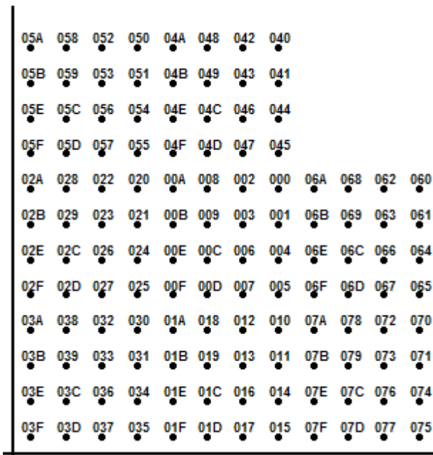
Figure 4-54: Constellation diagram for 512QAM (NATURAL, SMx), including the logical symbol mapping (hexadecimal); the figure shows the upper right section of the diagram only
