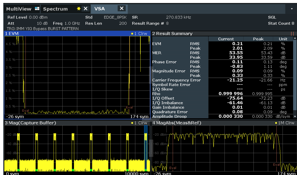
Figure 9-8: Result range that exceeds the burst length
