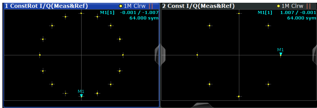
Figure 3-5: Result display "Constellation I/Q (Rotated)" vs. common "Constellation I/Q" for 3\pi/8 -8PSK modulation
