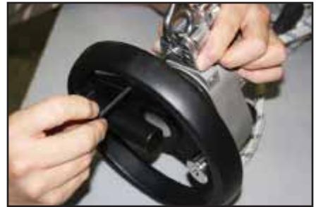
Step 3 - While holding the adapter and plate in place, insert the two screws and tighten until snug.
