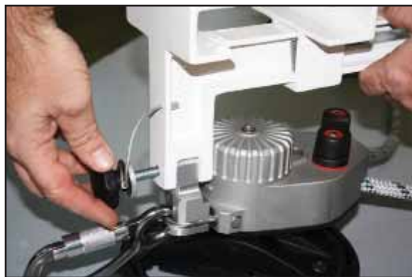
Step 5 - Insert the pin and tighten completely, ensuring that the pin extends through both holes in the ladder bracket.
