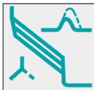
Molded case circuit breaker characteristic curve for motor protection with adjustable trip class ETU40M
