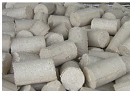
Briquettes made from sawdust left over from the piano manufacturing process (pellet)
