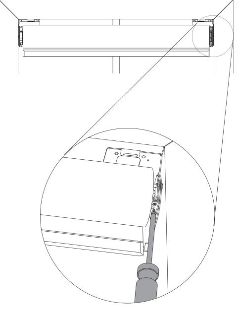
Plug 4-pin terminal block on cable into EDU terminal block.
