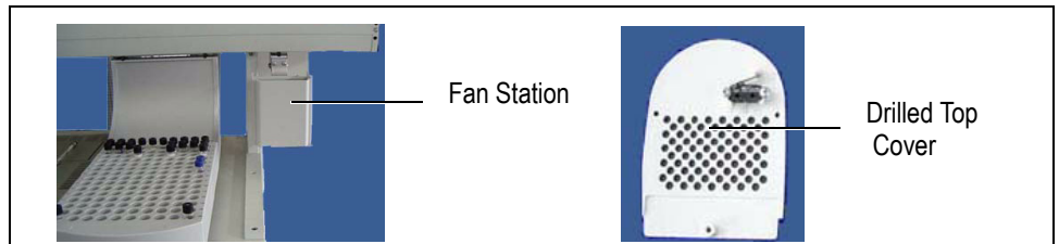
Figure 4-36. Example of Fan Station Installation
