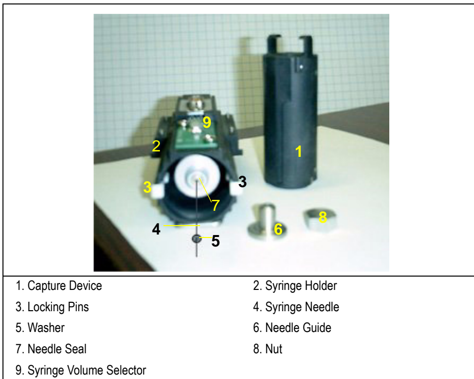
Figure 2-13. HS Injection Device Components
