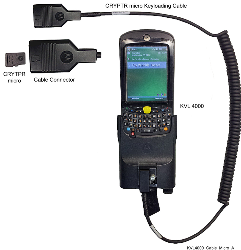
Figure 3: KVL 4000 Model T7537B with CRYPTR micro Keyloading Cable
