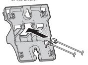
Tuck the telephone line cord inside the wall mounting adaptor (1). Connect the AC adaptor cord and telephone line cord (2).
