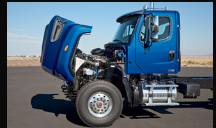
Full tilt hood for easy engine access.
