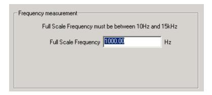
You can enter any frequency between 10 Hz and 15000 Hz as full scale frequency. LMA-3 measures the frequency with a resolution of 0.1 % of the full scale frequency specified. So in LogWorks 0 Hz is always 0 Volt, and the full-scale frequency is equivalent to 5 Volt. This functionality is also available for Inputs 4 and 5.
