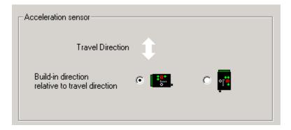
Select the travel direction of the car. Please note that changing this setting will effect the travel direction setting for side force measurements on Input 2 as well.
