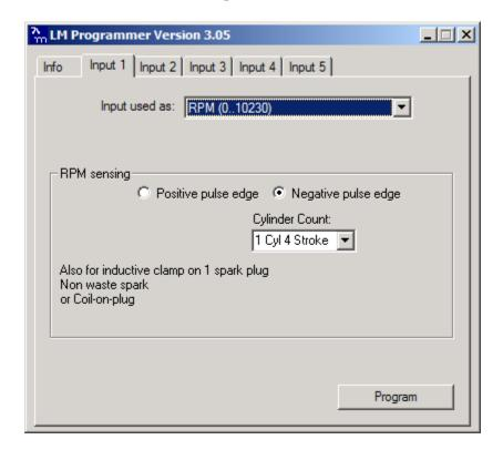
The drop-down list at the top of the window allows you to select the different functionality for that input. If RPM is selected, the area below the functionality selection shows as above.
