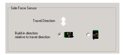
Select the travel direction of the car. Please note that changing this setting will effect the travel direction setting for acceleration measurements on Input 5 as well.
