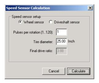
Select if you use a drive-shaft sensor or a wheel sensor. Enter the pulses per rotation created by the sensor either as driveshaft rotation or wheel rotation. You also need to enter the wheel diameter, and in case of a drive-shaft sensor, the final drive (differential) ratio.
