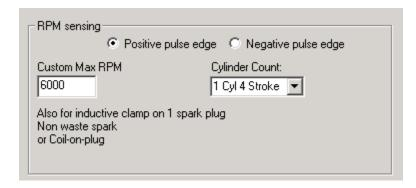
On the left edit box you can specify the max RPM for this measurement channel. In the example case the max RPM is 6000. This means that in LogWorks 6000 RPM is equivalent to 5Volt. This allows LogWorks to have a higher RPM resolution (~ 6 RPM per step instead of 10 RPM when the range is 0..10230 RPM). This functionality is also available for Inputs 4 and 5.
