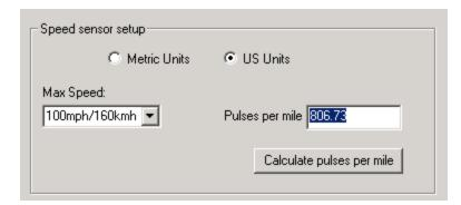
With the radio buttons you can select to use metric (km/h) or US (mph) units. In the left drop-down list you select the max speed to be measured. The LMA-3 measures the speed with a resolution of 0.1 % of the selected max speed.
