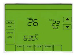
on. "WAIT" will now disappear and "COOL ON" will appear. (Note: on some systems there could be a 10-15 minute delay). Once you hear the compressor fan running, you should feel cool air at the vent. Once you have confirmed the system is operational, set the thermostat to a higher desired temperature to conserve energy. (ex. 26C or 79F)
