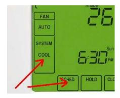
2. Temporarily set the temperature below the current room temperature displayed on the thermostat (ex. 23C). "WAIT" will show just below the "SET TO" temperature display.
