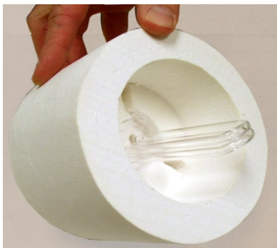
Figure 8-16. Pyrolyzer tube inserted into the insulation
