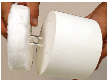
Figure 8-17. Apply the Kaowool insulation
