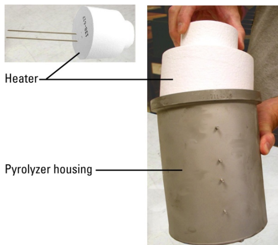
Figure 8-7. Insert replacement heater into housing
