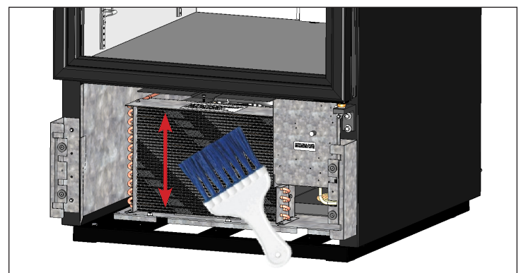
Fig. 4. Never brush across the coil fins.
