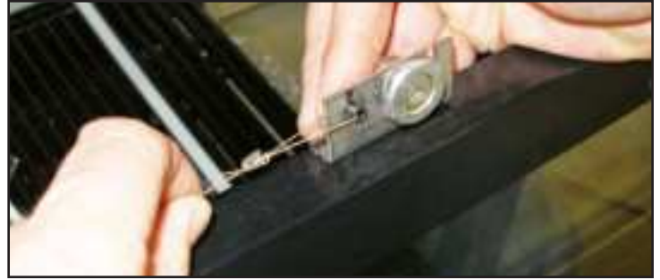
Fig. 7. Remove the door cord from the roller bracket.
