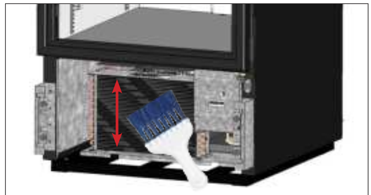
Fig. 4. Never brush across the coil fins.
