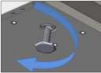
Fig. 1. Turn the leveling legs clockwise to lower the unit.
