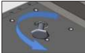
Fig. 2. Turn the leveling legs counterclockwise to raise the unit.
