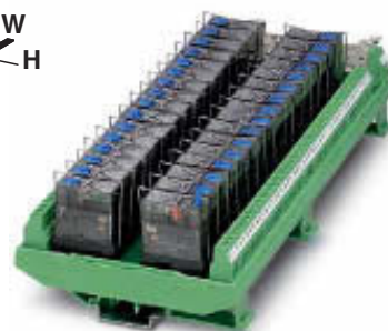
Output module with 32 miniature relays, 1 PDT with detectable manual operation
