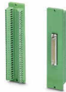
With high-density D-subminiature pin strip
