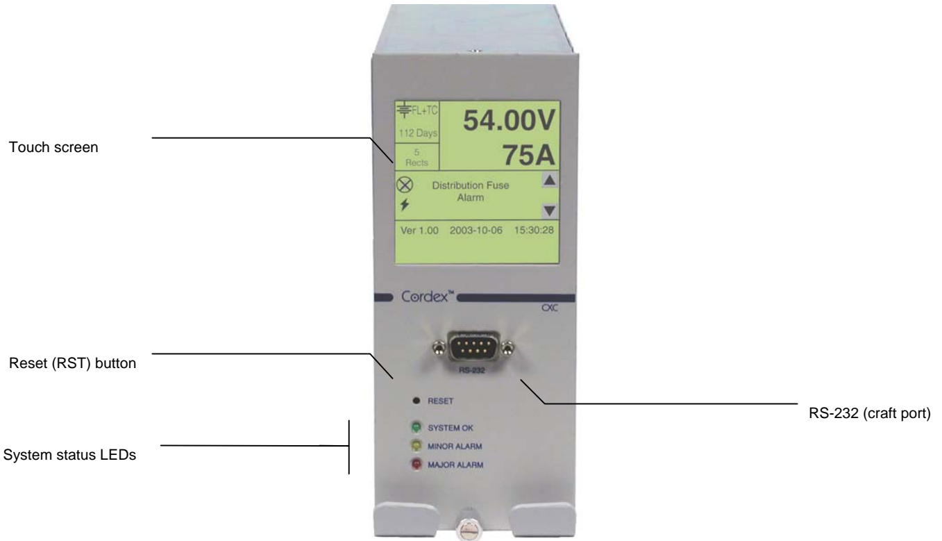
Figure 4–Cordex CXCM model system controller front panel
