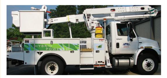
This fall, PWC will introduce their first hybrid bucket trucks into its fleet. Using a Jobsite Energy Management System, the hybrid is designed to fully operate its lift on battery power.
