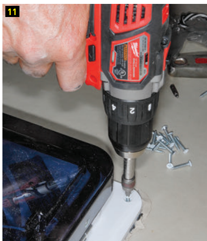
(9) A foam gasket is applied to the Fan-Tastic Vent before it is positioned (10) into the hole in the roof. No other sealant is needed on the gasket surface. (11) Once it has been established that the fit is correct (from the inside) and the shroud slides into place without restriction, it's time to attach the new vent to the roof using the supplied screws. (12) Lap sealer is applied around the edges of the Fan-Tastic Vent frame and on the screw heads. Lap sealer fills voids as it spreads. It takes a little practice to apply the right amount of sealer; in most cases, more is not better.
