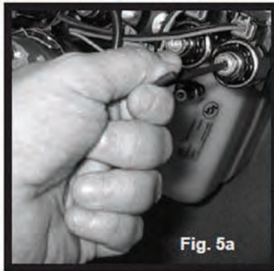
Clockwise for manual override
