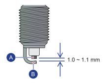
After cleaning and checking the gap, reinstall the spark plug and tighten by hand to avoid cross threading. Finally tighten using spark plug spanner.
