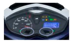
The multifunction display of the speedometer has various functions like 'ODO', 'TRIP A', 'TRIP B', 'TRIP F#', 'DTE##', 'AFE', 'IFE' and 'CLOCK'.
