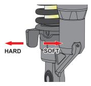
Adjust the spring pre-load by shifting the adjuster to the required notch according to the different load conditions. The more you compress the spring, the suspension becomes more stiff.
