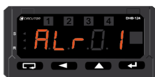
Figure 33:Alarm relay 1 configuration screen.
