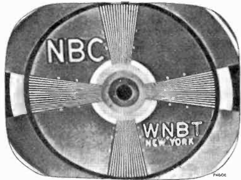
Figure 22—Horizontal Linearity Control Misadjusted (Picture Cramped in Middle)
