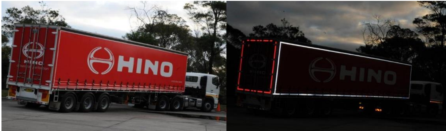
Figure 4.18 Visual effectiveness of conspicuity markings at night 37
