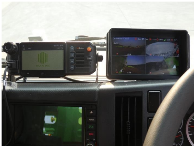
Figure 4.10 Example of blind spot camera on inside of a truck - Image courtesy of Sydney Metro.
