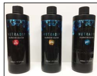
TDS 1000 EC ppm solution: To calibrate total dissolved solids probe
