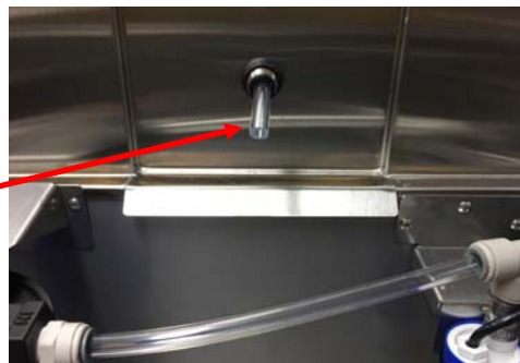
Fig. 5 Zone irrigation nozzle
