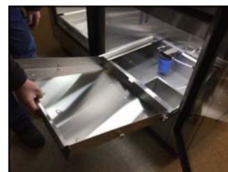
Fig. 1 Access the water reservoir; the sensor will be on the left side
