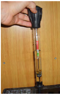
77-200-00: Hydrometer Used for testing battery electrolyte. Illustration is of a typical hydrometer, actual hydrometer type may vary.
