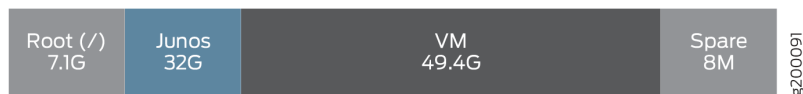
Figure 8: Host partition table for Routing Engines on MX2010 and MX2020 routers with 100GB SSD
