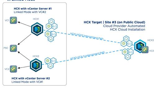
• The resulting behavior is that HCX operations for the combined inventory can be initiated from any of the vCenter Servers that are in Linked Mode.
