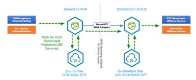
The HCX-WAN-OPT automatically uses the Management Network segment configured during the HCX-WAN-IX deployment. It is auto-assigned special use HCX internal RFC-5735 addresses for communications with the HCX-WAN-IX.
