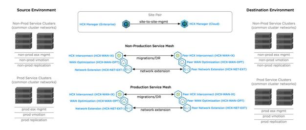
Alternatively, if in this example all Prod and Non-Prod have common cluster networks, the production and non-production Service Clusters can be added later to a single compute profile:
