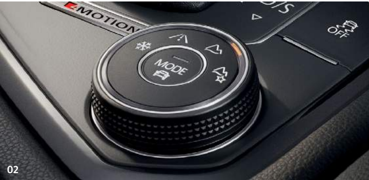
02 All 4MOTION models feature 4MOTION Active Control which allows you to adapt your Tiguan to suit the weather and road conditions ahead. Choose from four driving modes including On road, Off-road, Off-road Individual and Snow, enabling you to find the optimum choice of driving mode wherever your adventures may take you. Standard on all 4MOTION models. Image shown features optional 'Vienna' leather upholstery.
