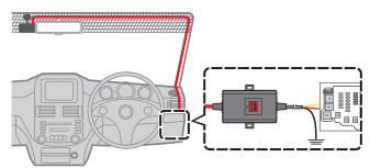
Connect the Smart Box II to the dash cam and confirm it is working properly by the LED indicator that glows in red. Then you can arrange the cable and complete the installation.
