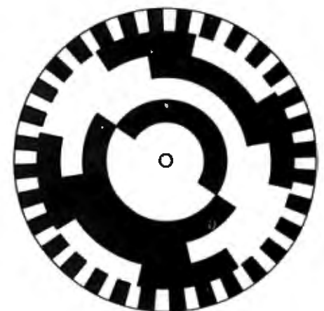
Figure 3: The optical encoding disc uses a Gray code to eliminate ambiguity in angular position of the wind vane, while in the anemometer only the outermost ring is used as a sort of tachometer.
