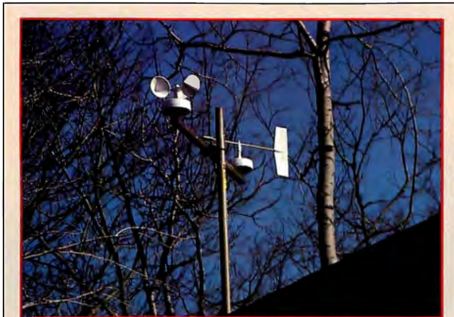
Photo 1: Wind-velocity measurements are taken by a cup anemometer and wind vane mounted high above any obstruction to air flow on a section of television-antenna mast.
