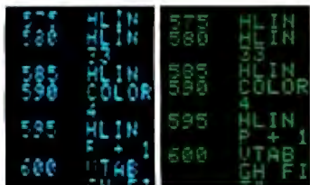
Compare display quality of a typical home TV (left) with a Sanyo professional monitor (right).
