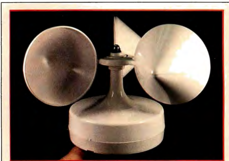
Photo 4: Completed Heathkit anemometer assembly.
