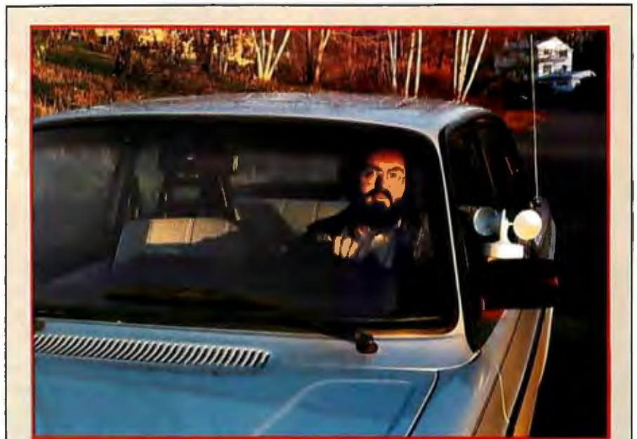
Photo 6: The anemometer was calibrated by moving it relative to still air; holding it out the window of a moving automobile worked quite well. Driving at a known speed, I used the circuit of figure 5 to record its pulses; the characteristic curve is shown in figure 6.
