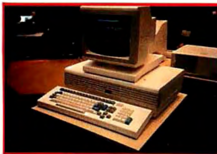
Photo 1: The Fortune 32:16 microcomputer with Motorola 68000 processor.
