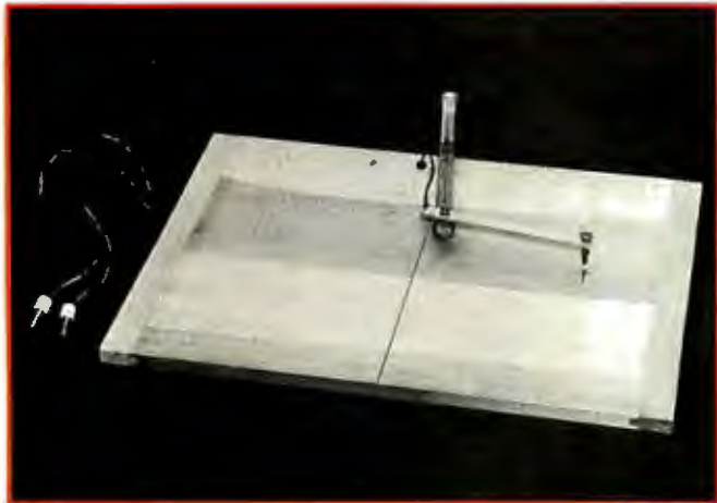
Photo 1: The homebrew graphics-tablet digitizer, built from a standard drafting table.
