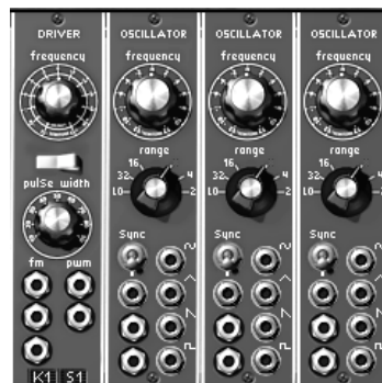
An oscillator bank: 1 "driver" and 3 "slave oscillators"
