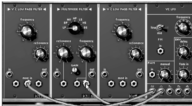
LFO1 to the filters link
