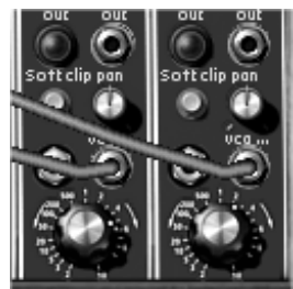
The connections to the two VCA
