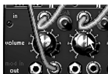
Setting of the volume of the 2 mixer VCA
