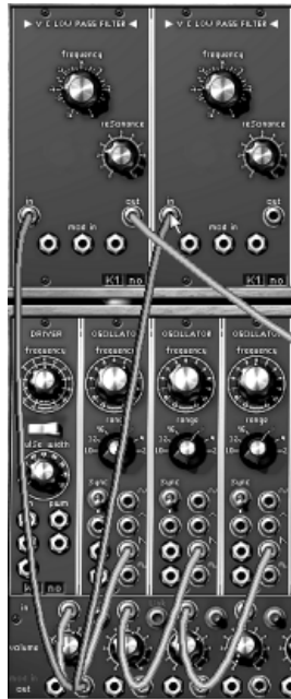
Connection towards the second filter
