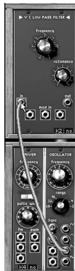
Connection between oscillator 1 and filter 1
