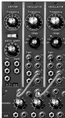
Connection of oscillators to mixer
