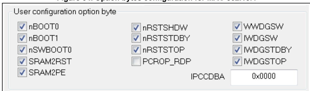
Figure 54. Option bytes configuration for MAC 802.15.4
