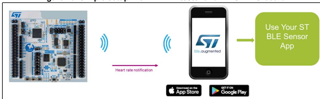
Figure 20. Simple setup with BLE RF tester and P-NUCLEO board
