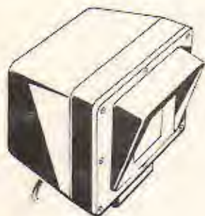
◀ Fig. 1. Traffic-light radar unit which uses microwave frequencies.
