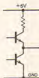
Fig. 4. T.t.l. output configuration leads to current spike at transmission.
