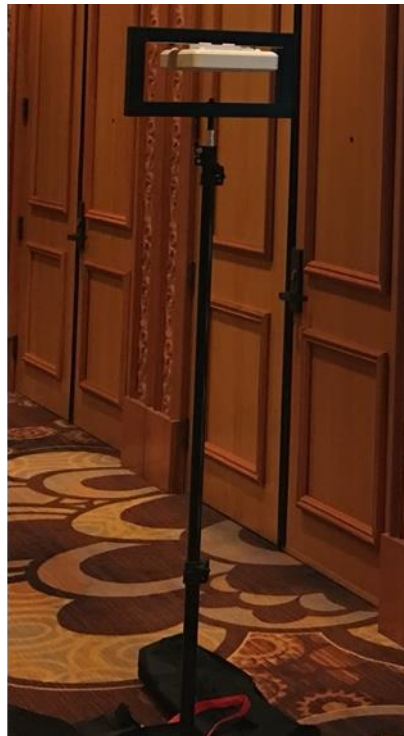
FIGURE 4: RUCKUS-DESIGNED SITE SURVEY STANDS ON TRIPODS
