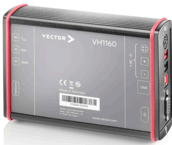
Compact VH1160 test hardware device for automating ECU conformance tests with CANoe.
