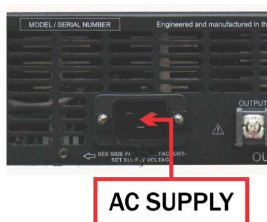
Figure 3.5 – Close-up of AC Mains Outlet
