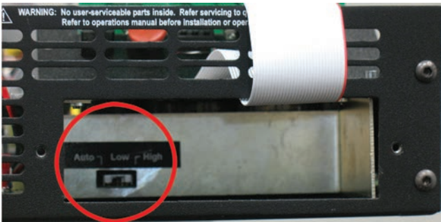
Figure 5.10 – Bi-Level Power Switch Location
