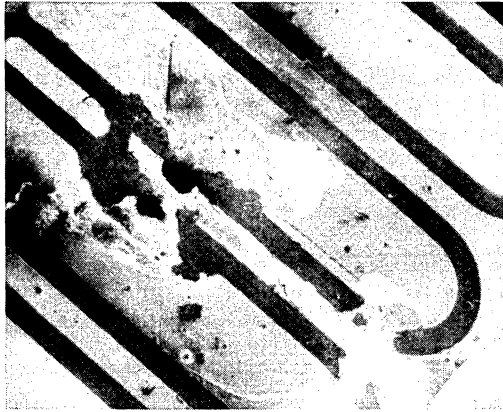
Figure 26. Photomicrograph of Damage Due to I_{s/b}
