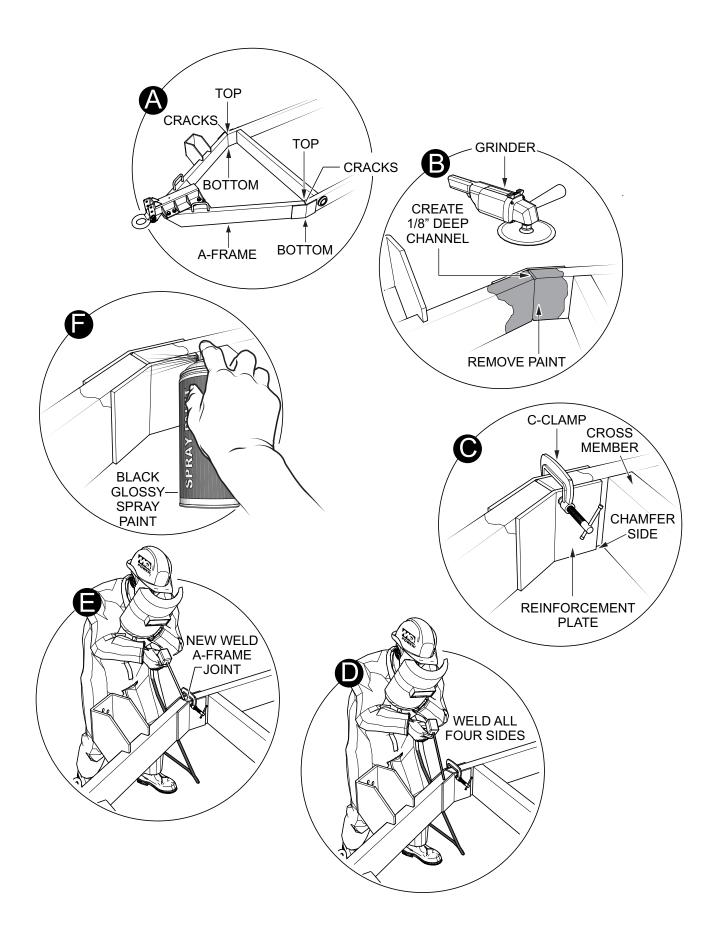
Figure 2. Inner Reinforcment Plate Installation
