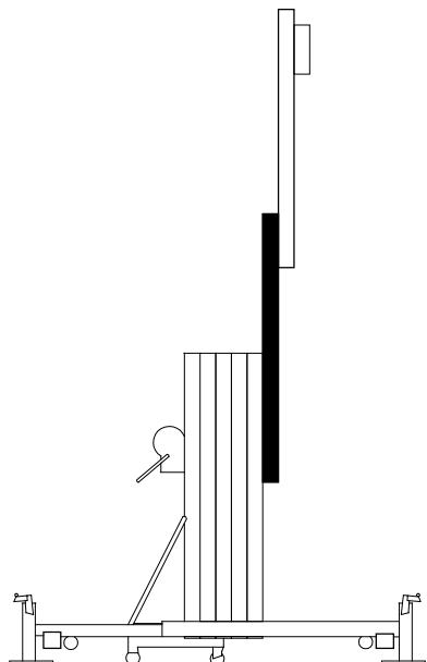
**▲ CAUTION** Crushing hazard. Do not stand directly under the columns or load handling attachment.
