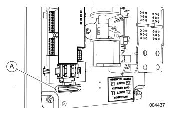
Figure 4-2. Fuse Removal and Installation Tool
