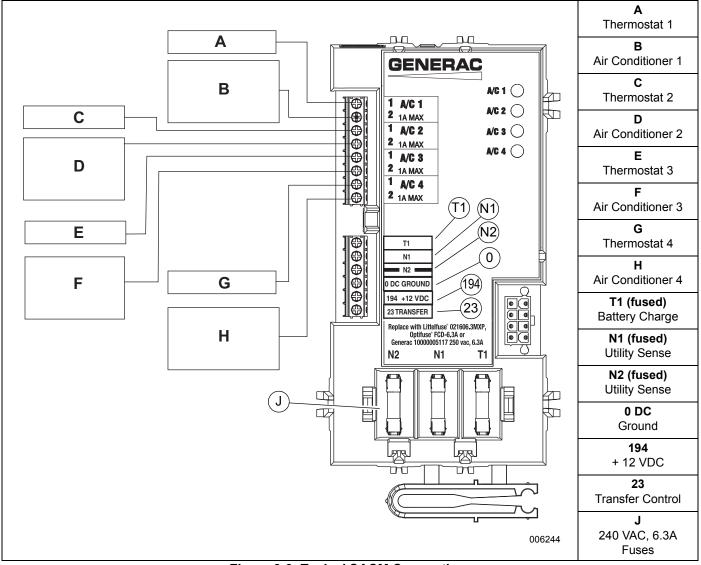
Figure 3-3. Typical SACM Connections
