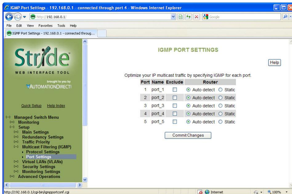
**Exclude:** A port may be excluded from IGMP processing. IGMP queries and reports received on an excluded port are ignored so devices reached via the excluded port cannot join multicast groups filtered by the switch. IGMP queries and reports will not be forwarded to the excluded port so IGMP routers reached via the excluded port will not know of memberships for devices reached by other ports.
