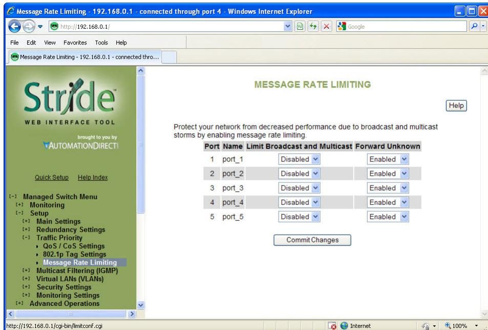
Limiting is done based on message type and priority. Broadcast and multicast messages are prioritized (by IP ToS) then limited to approximately the following rates:
