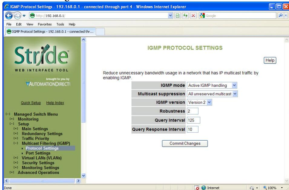
The default settings will allow the switch to recognize members of a multicast group and forward the multicast message to only members of that group.
