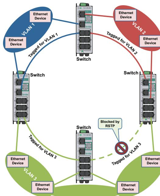
The solution to the problem above is to configure all “Network” type ports to carry all VLANs in the network. In other words, the Network Port should be a member of all VLANs defined in the switch. As seen from the example shown in the following diagram, VLAN 3 can forward to all its members through the other Network Port connections and is not affected by the block RSTP connection.
