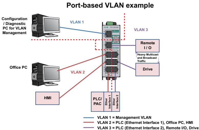
**Solution:** We will use a Stride managed switch, utilizing the Port-based VLAN feature. The question could be posed, “Why not just use two unmanaged switches?” While this would work, the customer wants to use as few components in the system as possible to minimize points for possible equipment faults and he would like the enhanced diagnostic capabilities that a managed switch provides.
