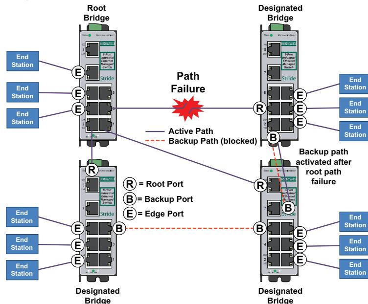
The Rapid Spanning Tree Protocol provides a standardized means for intelligent switches (also called bridges) to enable or disable network paths so there are no loops, but there is an alternative path if it is needed. Why is it called Rapid Spanning Tree Protocol?
