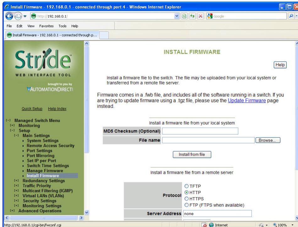
Firmware may be directly uploaded to the switch from the local system.
