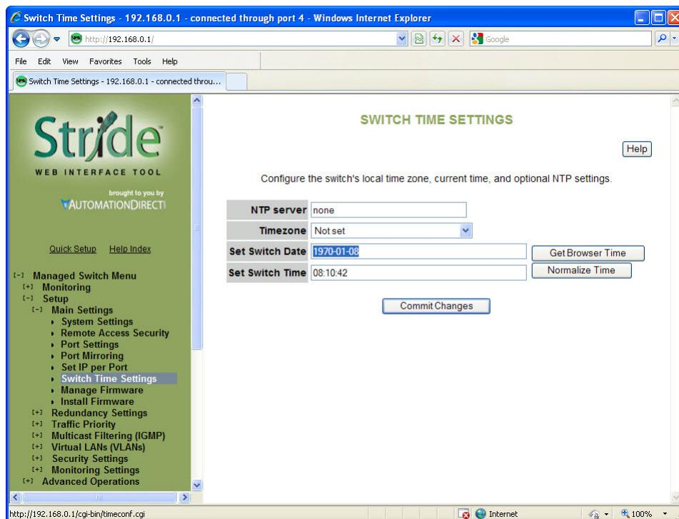
**NTP server:** You may specify an NTP server to automatically set the switch's clock. If a DNS server is configured, you may use a fully qualified domain name; otherwise, you must specify an IP address.
