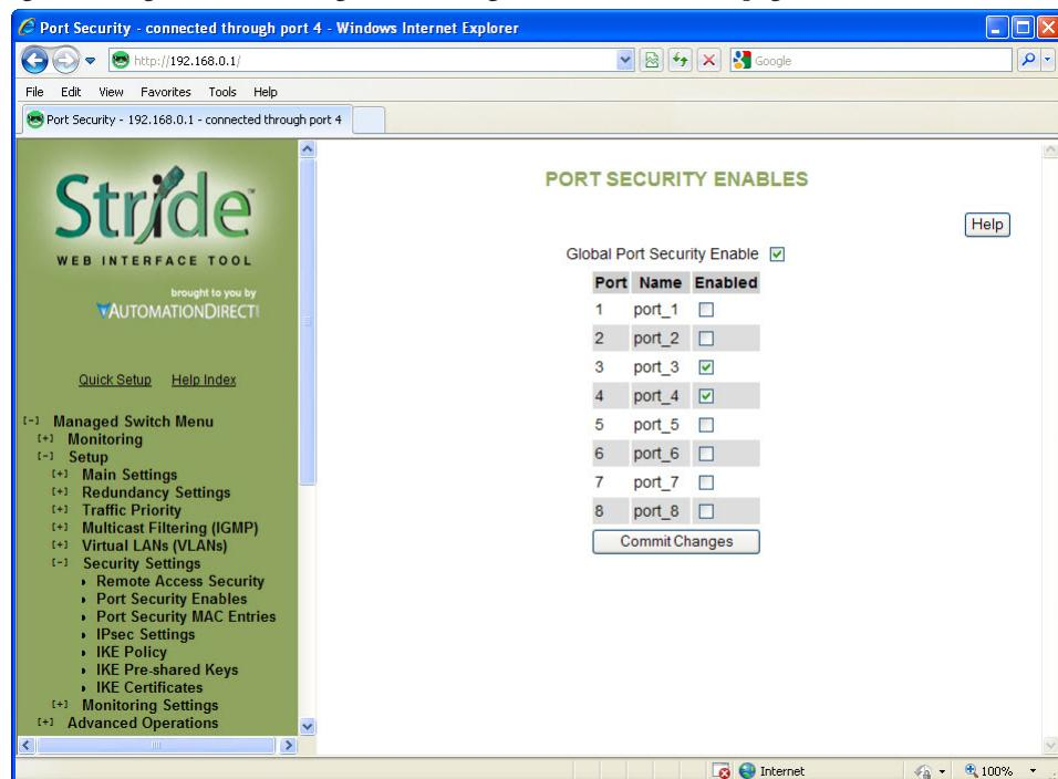
Once an entry has been configured and committed to the switch, a power cycle will be necessary after deletion of an entry in order for that security to be removed.
