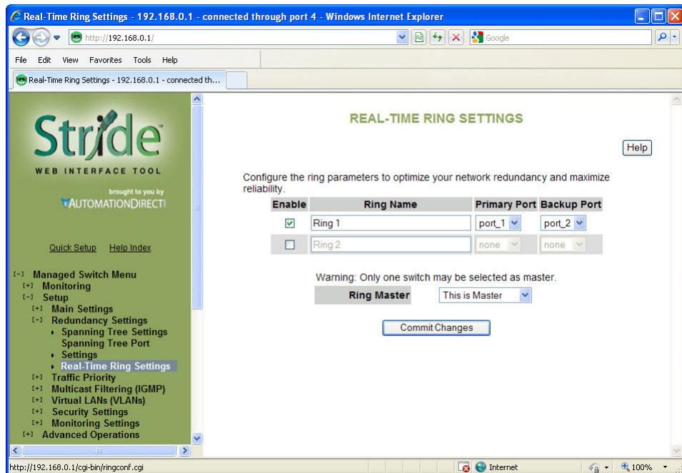
Activate a ring by selecting the appropriate Enable check box. You can configure one ring for every two ports on the switch.
