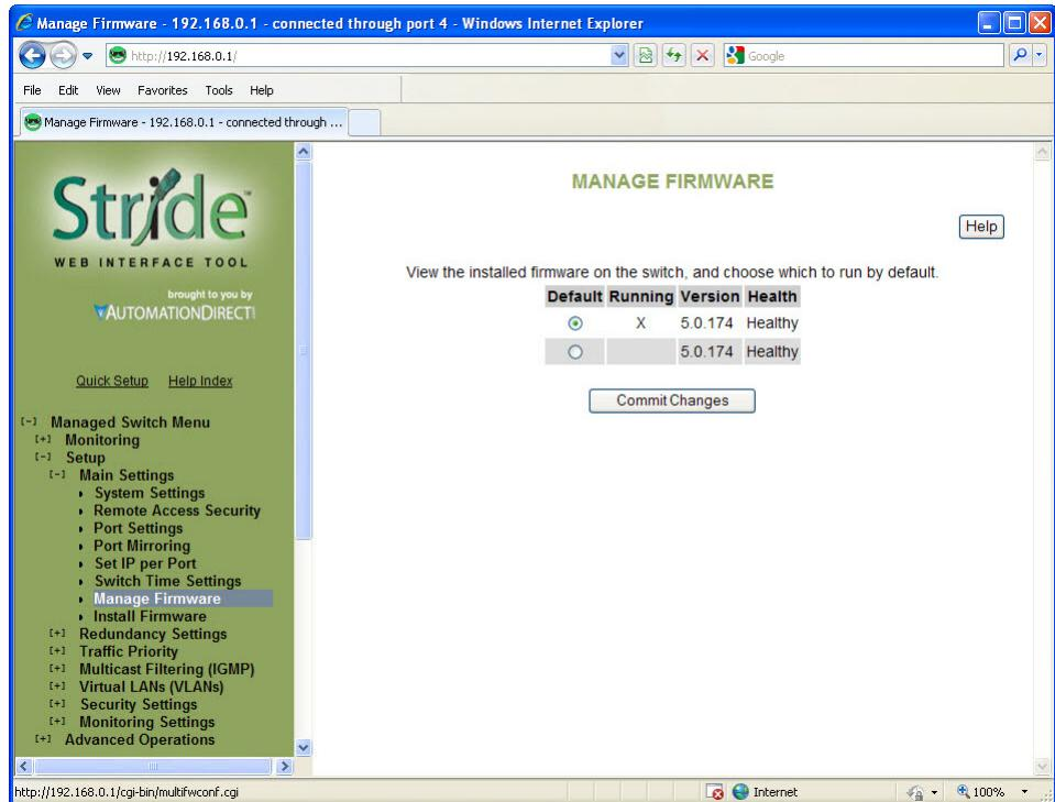
**Default:** Shows the current default firmware image to run when the switch is reset. May be changed to run a different firmware on the next reset.
