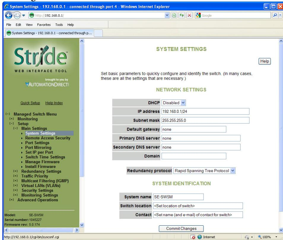
To control and monitor the switch via the network, it must be configured with basic network settings, including an IP address and subnet mask. Refer to the quick start guide in Chapter 2 to learn how to initially access your switch.
