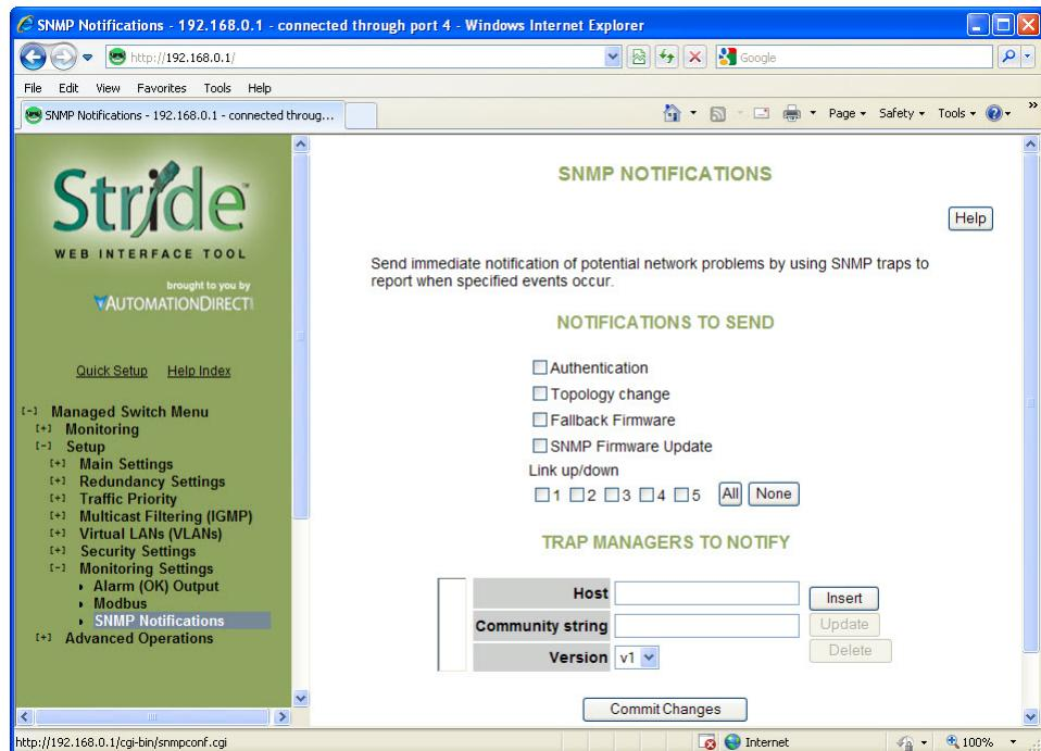
Use the SNMP Notifications Menu to enable traps to be sent when the state of the switch changes. Access this menu by selecting Setup from the Main Menu, and then selecting Main Settings.
