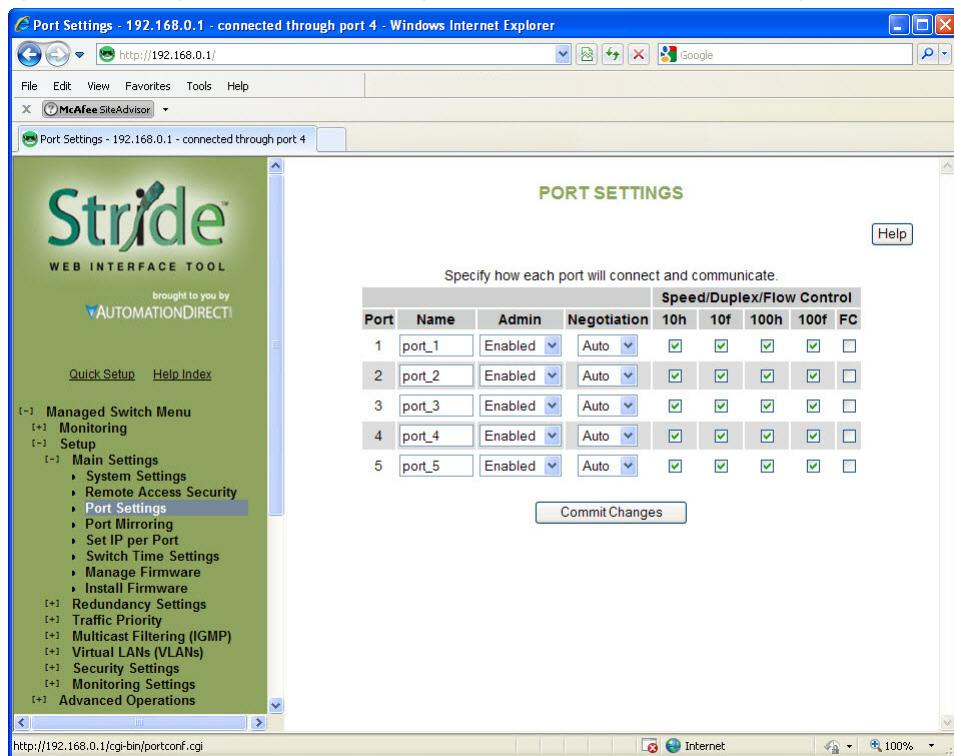
**Port Name:** Each port in the managed switch can be identified with a custom name. Specify a name for each port here.
