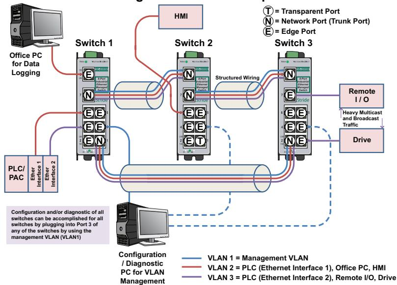
**Solution:** Use Stride managed switches, utilizing the VLAN feature to separate the broadcast and multicast traffic from all the devices except for the PLC. We will also wire the three switches into a Ring configuration so that we can take advantage of the redundancy feature of the switch. In this situation, we need to use Tag-based VLANs since the Ethernet packets will be traversing across multiple switches.
