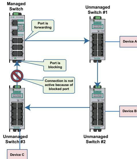
Initially, everything is working fine in the network. The managed switch detects the loop by seeing its own configuration messages and based on STP parameters, chooses one port to be in the forwarding state, and the other port to be in the blocking state. No loop is formed and device A can talk to device B.
