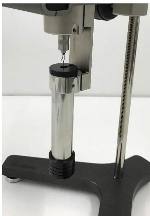
Fig.8: LCP Adapter assembled in viscometer
