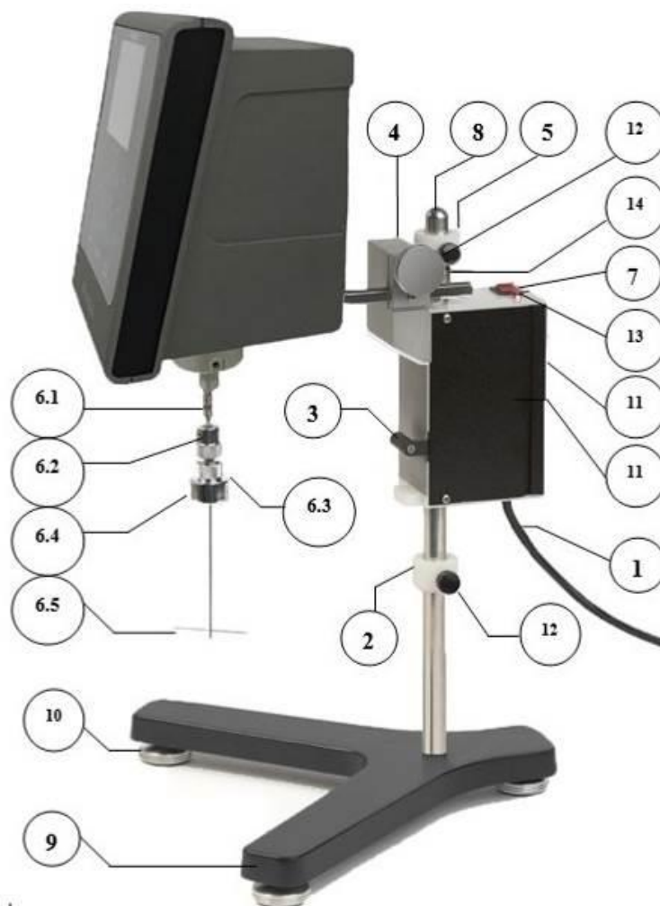
Fig. 17 Haldal unit set in the viscometer
