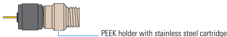
Figure 70. Column Out line connected to the deeper end of the PEEK holder
