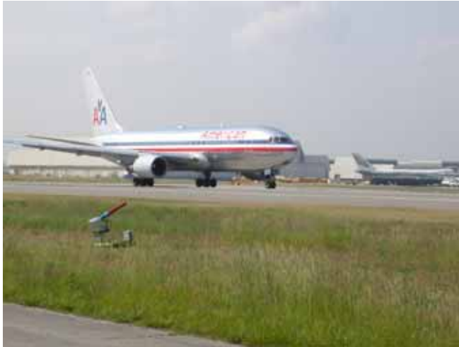
Propane cannons can be used as part of an integrated program to disperse birds from airports. However, birds quickly habituate to the loud bangs if the cannons are used continuously and not integrated with other frightening devices (photo by R. A. Dolbeer, USDA).
