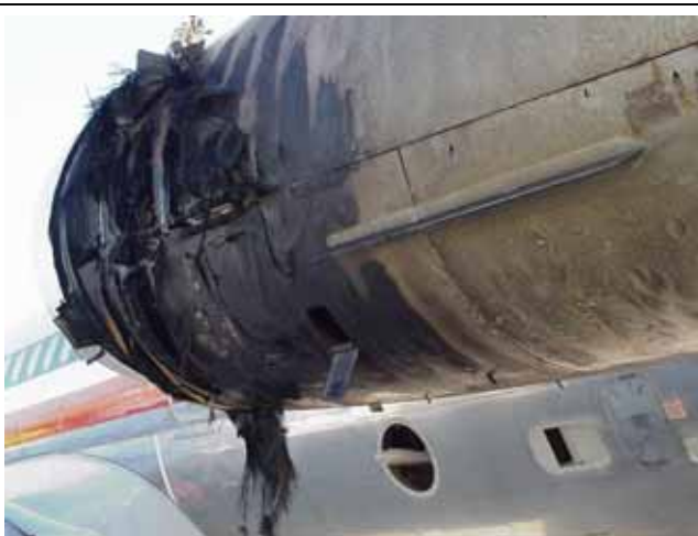
This is the #1 engine of the MD-80 after ingesting at least 1 double-crested cormorant on 16 September 2004. (See story on page 22.)
