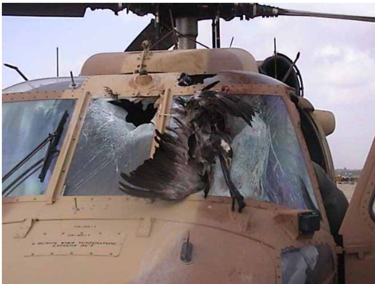
A Eurasian crane penetrated the windshield of this Israeli helicopter in March 2003. In the USA, vultures and waterfowl have been responsible for the most losses of military aircraft to bird strikes.
