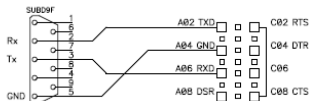
Figure 82. Cable wiring for BusinessPhone
