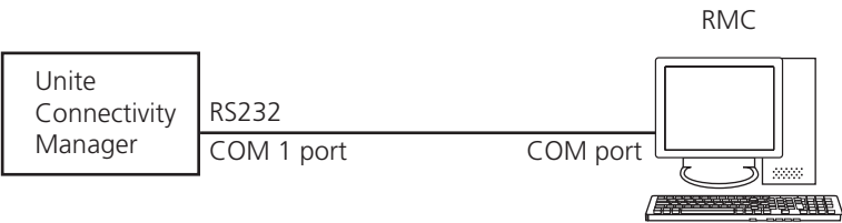
Figure 85. Connection for Remote Management.
