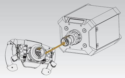
Pull and hold the Quick Release sleeve and carefully push the steering wheel onto the shaft.
