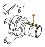
Centre the DD2's Quick Release shaft so that the slot is facing up.
