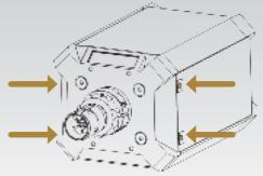
IMPORTANT: Use only good quality M8 bolts. Choose the bolt length so that the thread does not reach more than 20 mm into the wheel base. Always use all four hard-mount points, this allows a proper and stable installation and avoids damage!
